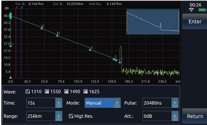
Figure 7-6 Test condition setting interface
