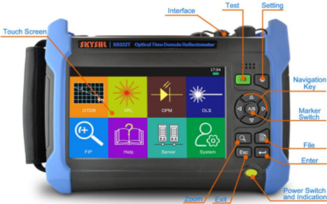
Figure 1-1 Front panel of optical time domain reflectometer
